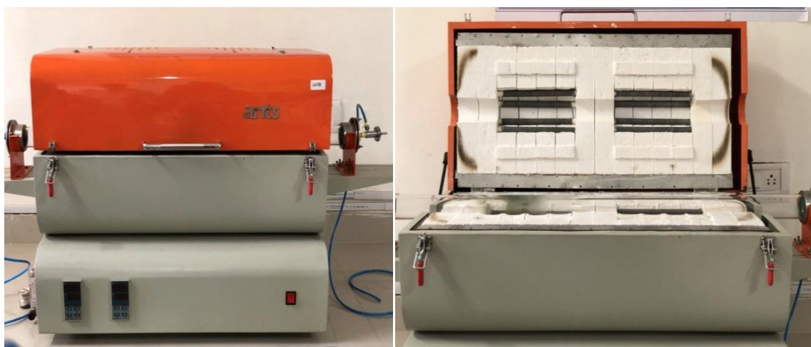
Figure 4.1. Thermal CVD equipment used for synthesis in laboratory.
