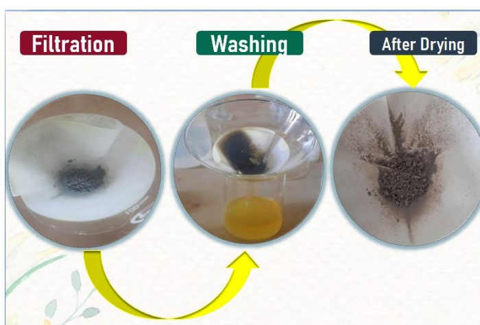
Figure 3.3 Extraction process for WS 2
